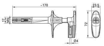
For fast and safe contacting to M5 threaded bolts, for example on motor connections (contact depth 3 to 6 mm). Ø 4 mm rigid socket in handle accepting spring-loaded Ø 4 mm plugs with rigid insulating sleeveThread inserts are replaceable and available separatelyThe current depends on the thread insert.
