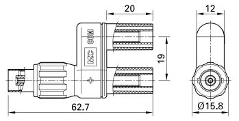
Two-pole touch-protected adapter with  $\varnothing$  4 mm connectors linked to the BNC system. Version with BNC female and rigid  $\varnothing$  4 mm sockets, accepting  $\varnothing$  4 mm plugs with rigid insulating sleeve. The contact socket of the inner conductor of the BNC connector is in gold-plated brass.
