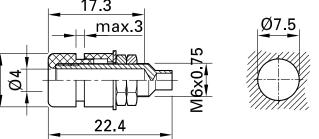
Insulated, Ø 4 mm, rigid. Machined brass. The socket can be screw-mounted in predrilled panels. Threaded bolt M6x0.75 and solder connection.
